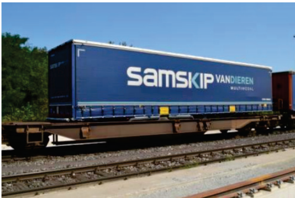
Image 1. Illustration of the huckepack technology SOURCE: http://baltictransportjournal.com/
