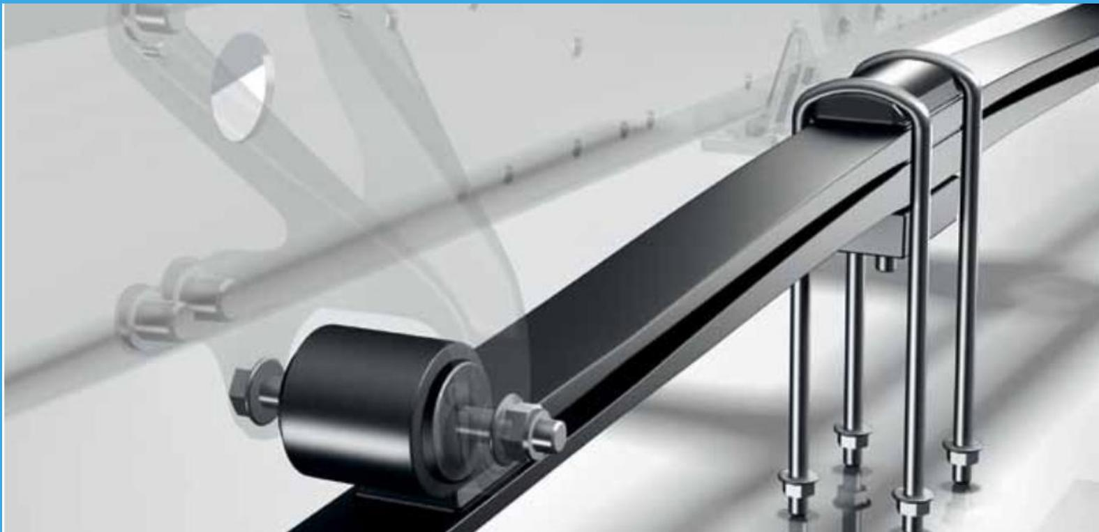
**Steel suspension.** For a high standard of ride and suspension comfort on- and off-road, the Atego is equipped with weight-optimised multi-leaf parabolic springs.
